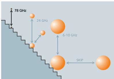
The higher the frequency of the radar transmitter, the more direct the signal reflection. Reliable measurement is thus guaranteed, even with large angles of repose.
