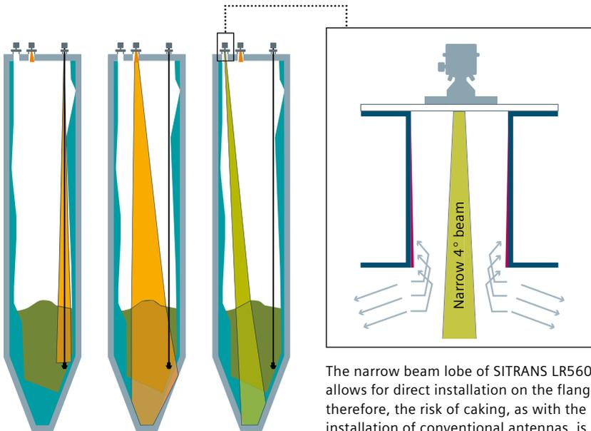
The narrow beam lobe of SITRANS LR560 allows for direct installation on the flange; therefore, the risk of caking, as with the installation of conventional antennas, is very low.
