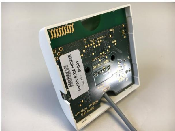
The housing cover with the latched circuit board and connected cable looks like this:
