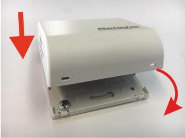
Finally, the housing cover incl. printed circuit board is clipped onto the already mounted mounting plate. To do this, attach the lid to the top edge of the mounting plate and press the lid firmly onto the plate until it snaps into place.
