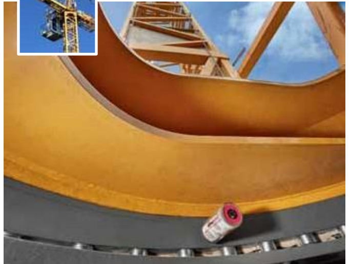
125 ml simalube lubricators lubricate the rotating assembly of a crane.
