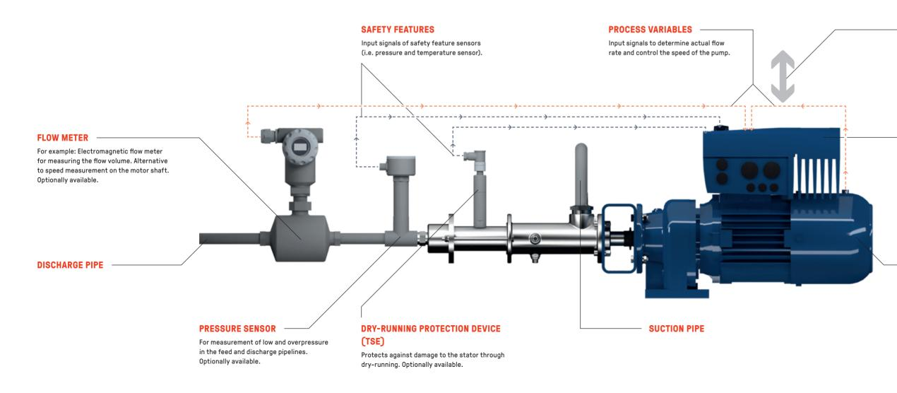
The SDP features an integrated PLC to enable stand alone operation in, for example, distributed control systems (DCS). Set points are entered and sensors on the pump feed back operating conditions to the integrated PLC. Complex implementation into higherlevel controllers is no longer required. This simplifies automation system integration and reduces the cost of installation and maintenance.
