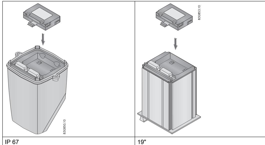
2. Press the add-on module in the direction shown until it stops and is firmly seated in position
