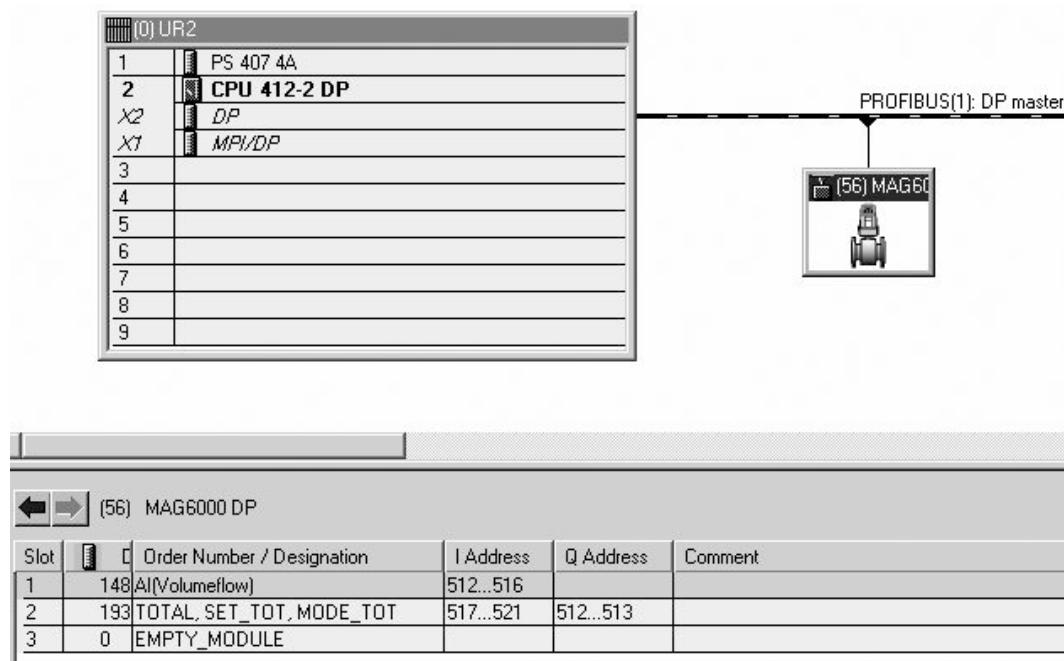
The next example shows Slot 3 being configured for using the Batch functionality on the transmitters digital output. The master sends Batch Control, Batch Setpoint and Batch Compensation to the flowmeter and receives batch amount and batch status from the flowmeter. In MAG6000 it is possible to assign the batch functionality to the digital output or to the relay output.
