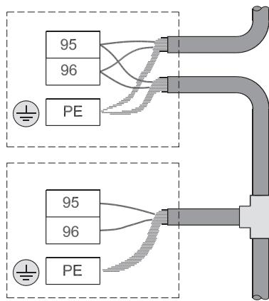
Figure 4-1 PA electrical connection
