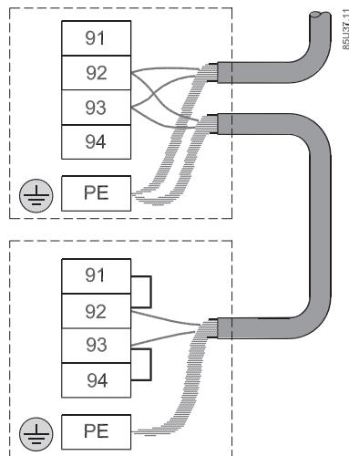
Figure 4-2 DP Electrical connection
