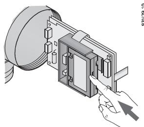
3. Reinsert the complete transmitter module
