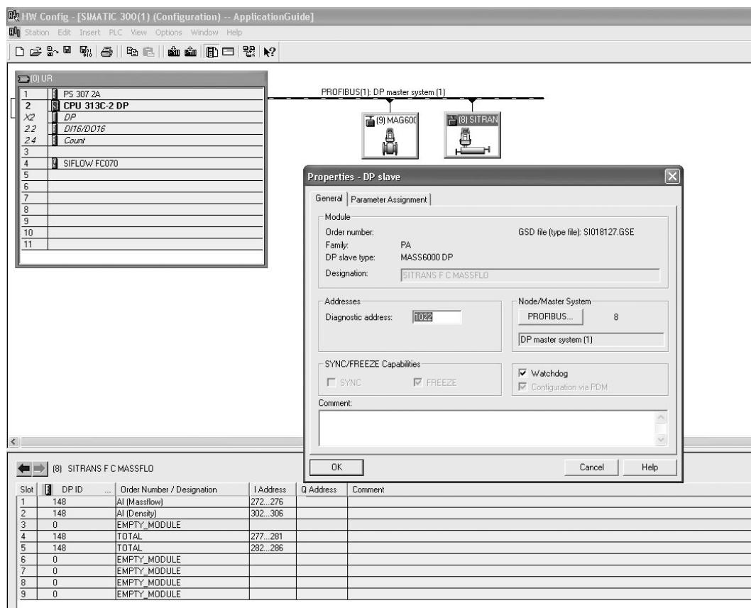
From this, we can see that if we wanted to address slot 0, LADDR would be W#16# 7FE (hex equivalent of 2046). If we wanted to address slot 1, LADDR would be W#16#100 (hex equivalent of 256).
