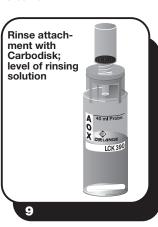
Any attached Carbodisk-fibres should be removed from the stopper of the Carbodisk-holder with a paper towel as necessary.
