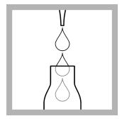
**1.** Pipette 1.0 mL of sample into the digestion cuvette.
