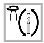
**12.** Close the cuvette and invert a few times until the freeze-dried contents are **completely dissolved**.
