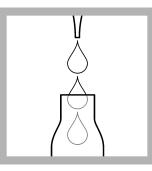
2. Pipet 0.5 mL Reagent B. Close Reagent B immediately after use.
