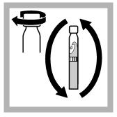
**4.** Close the cuvette and invert a few times until the freeze-dried contents are **completely dissolved**.
