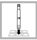
6. Heat in the thermostat. HT 200 S: in the standard program HT for 15 minutes.
