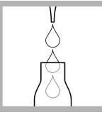
**10.** Pipet into the cooled cuvette: **0.2 mL Reagent B**. Close Reagent B **immediately** after use.
