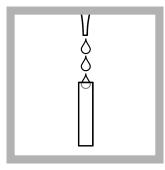
**2.** Pipet the iso-octane into the clean quartz-glass cuvette.
