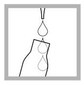
1. Run a 1-mL sample slowly along the length of the cuvette wall, in order to deposite the iso-octane phase cleanly at the buttom.
