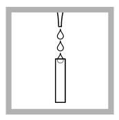
**2.** Use the pipet to dispense the organic phase into the quartz-glass cuvette.
