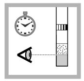
**6.** Let the contents of the cuvette settle for **1 minute** to ensure that the phase has fully separated.
