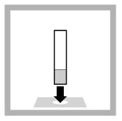
**4.** Insert the quartz-glass cuvette into the cell holder. DR 5000/DR 6000: Go to Stored programs. Select the test, push **ZERO**.
