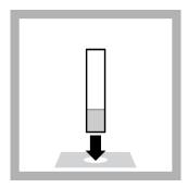
**4.** Insert the quartz-glass cuvette into the cellholder. DR 5000/DR 6000: Push **READ**.
