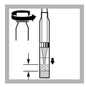
1. Remove the organic phase with up to 1 cm clearance using a Pasteur pipet.
