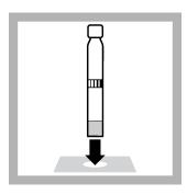
5. Insert the first sample cuvette (blank value). DR1900 / DR2800 / DR3800 / DR5000: push READ. Enter the number of samples and push OK. Insert the specified number of sample cuvettes. DR1900 / DR2800 / DR3800 / DR5000: push READ.
