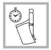
**8.** After **1 minute** thoroughly clean the outside of the cuvette(s).
