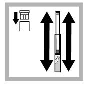
7. Place the rubber stopper on the filter plunger and shake until the precipitate is completely dissolved. This may take from just a few seconds to 5 minutes, depending on the sample.
