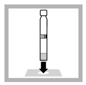
9. Insert the sample cuvette(s) (main value). DR1900 / DR2800 / DR3800 / DR5000: push READ. After the final sample cuvette has been measured, an audible signal is emitted.
