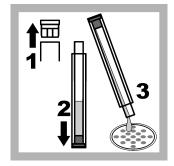
4. Remove the stopper from the filter plunger. Push the filter plunger down until it reaches the bottom of the plastic tube. Dispose of reacted solutions according to local, state and federal regulations.
