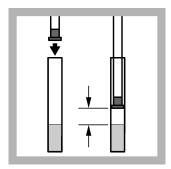
2. Place the filter plunger on the tube and push the plunger down until it is approximately 2 cm above the surface of the liquid.
