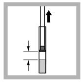
**6.** Draw filter plunger upward until it is approximately **2 cm** above the surface of the liquid.
