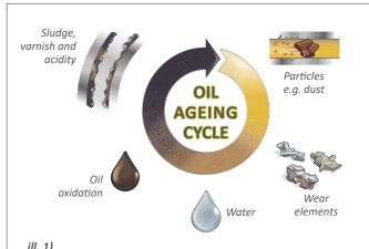
CIC® Filter Inserts remove all catalyst in the "oil ageing cycle" and will slow down the oil degradation process. If contaminants are not removed, a vicious circle starts and the oil degradation
