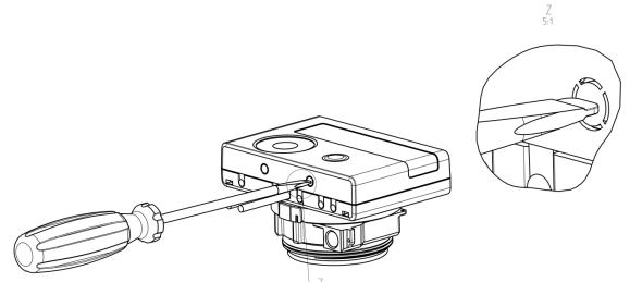
Then insert the screwdriver into one of the two openings at an angle of approx. 45° and carefully lift the handle up to approx. 90° (see picture 2). The upper housing piece of the calculator is then no longer latched on this side. Repeat this with the other opening. Now the upper housing piece can be taken off.
