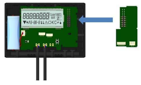
To remove a module the upper housing piece must be carefully pressed against the rear panel of the lower housing piece during opening the calculator. Thus the two rear snap-fits of the upper housing piece lever out the module of the PC board (see picture 4).
