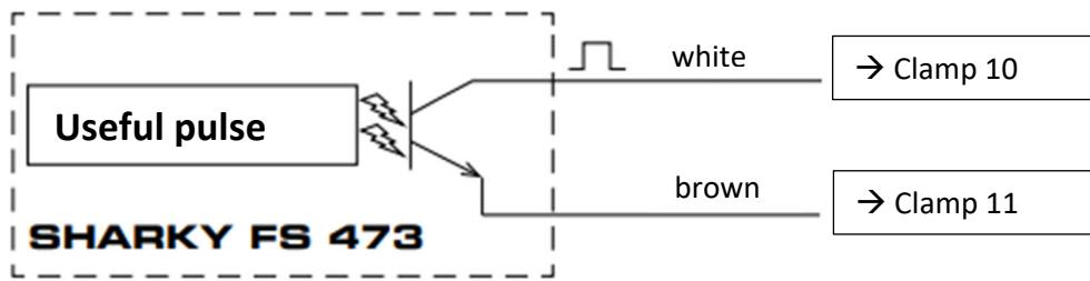
**Important note:** The colored marking of the cables corresponds to the scheme shown above.
