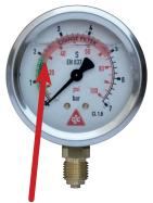
CJC™ Pressure Gauge <u>WITH</u> the sticker indicating when to change the CJC™ Filter Insert
